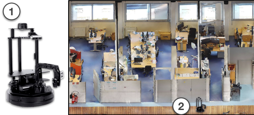
Figure 5.3 – The capture of real-world images are carried by an embedded RGB-D camera on a “Locobot” [150] ①. On the right ② such a robot is displayed with respect to proportions in its environment.
